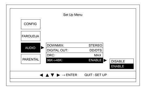
Press the  $\blacktriangledown$  button or key to choose the preferred sample rate option, then press the enter button or key.
