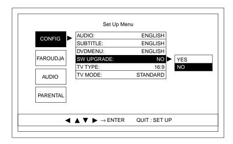
If you need to install an upgrade disc, press the ▶ button or key to select YES and press the enter button or key.
