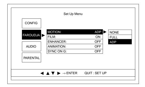
Press the ▼ button or key to choose the preferred motion compensation option, then press the enter button or key.
