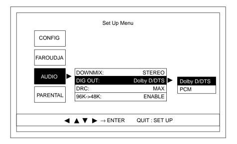
Press the ▼ button or key to choose the preferred digital output option, then press the enter button or key.
