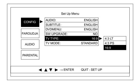
Press the  $\blacktriangledown$  button or key to choose the television type, then press the enter button or key.
